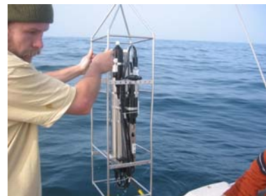
Fig. 6: CTDO deployment off Chipana.
